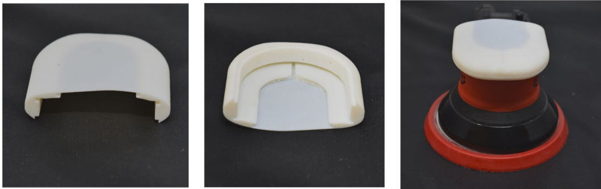
Figure 5: The sliding design for attaching to the sander.
