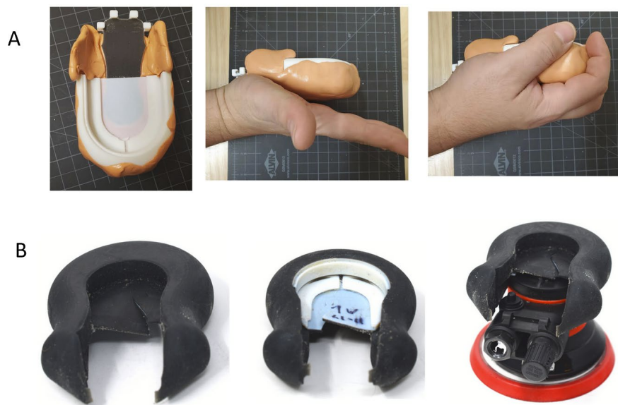
Figure 7: The grip was redesigned from concept (A) to initial design (B) to be more of a mushroom style grip.
