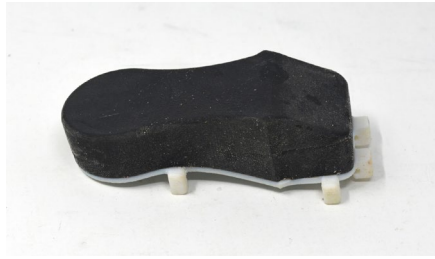
Figure 6: The claps for attaching to the lever pad of the gripper.
