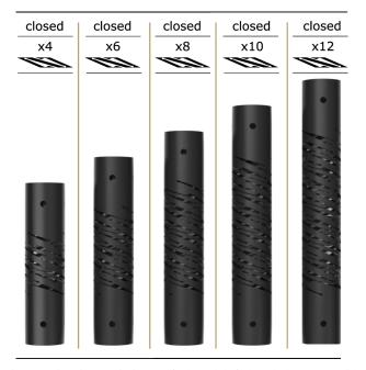
Fig. 3: Five instantiations of closed left-handed HSAs with varying row tilings from four to twelve. These are made by vertically stacking the closed pattern around a unit cell. *A. Mechanical Characterization*
